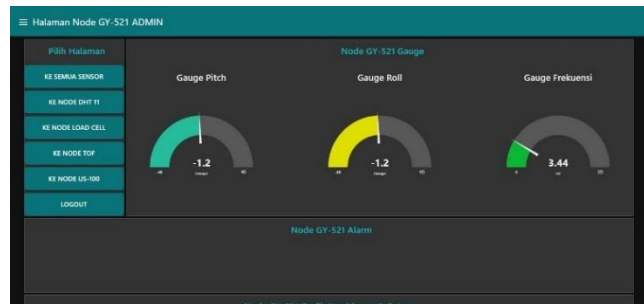
Gambar 6 Tampilan dashboard node GY-521
