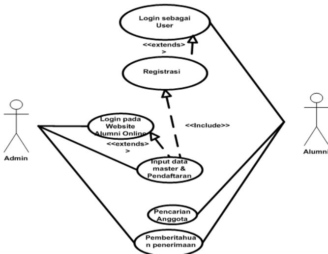
Gambar 3 Diagram use case sistem informasi *database* alumni
