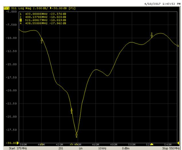
Gambar 16 Hasil *return loss* Antena1
