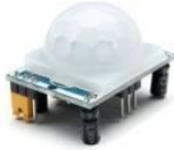
Gambar 3 Modul HC-SR501 Sumber: henrysbench.capnfatz.com/henrys-bench/arduino-sensors-and-input/arduino-hc-sr501-motion-sensor-tutorial
