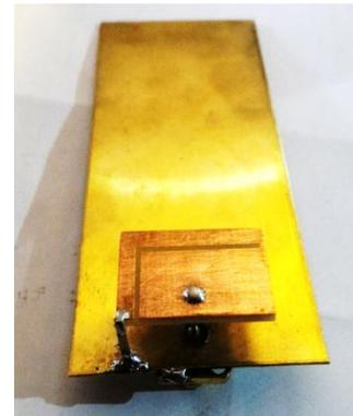
Gambar 10 Prototipe PIFA *L-slot*
